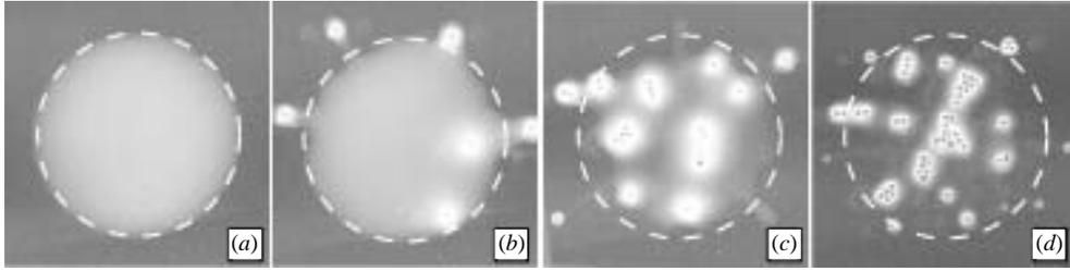
FIGURE 5. Photographs of droplets impacting at the same velocity  $U = 2.15 \text{ m s}^{-1}$ : (a) Liquid L2 without particles (b) Liquid L2 without particles at  $\phi = 0.04$ , (c)  $\phi = 0.13$  and (d)  $\phi = 0.30$ . Pure liquid Reynolds number is  $Re_0 = 8217$ .
