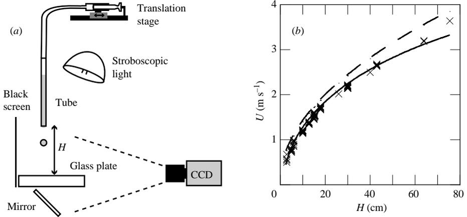
FIGURE 1. (a) Schematic diagram of the experimental apparatus. (b) Correlation between the height of release  $H$  and the impact velocity  $U$ . The dashed line is the free-fall velocity and the continuous line is the velocity obtained with  $U = \sqrt{gH_0(1 - \exp(-2(H - \Delta H)/H_0))}$ .
