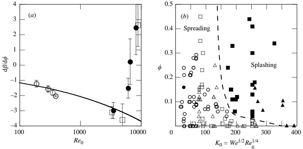
FIGURE 4. (a) Spreading reduction due to the particles L1P1 (open circles), L2P2 (filled circles) and L2P3 (squares). The continuous line is (2.5) computed with  $\phi_m = 0.68$ ,  $n = 1.87$  and  $\alpha = 1$ . (b) Map of the spreading/splashing regimes in the  $(K_0, \phi)$ -plane: L1P1 (circles), L2P2 (squares) and L2P3 (triangles).
