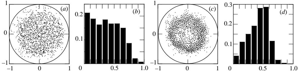
FIGURE 6. (a) Particle position distribution in the spread droplet and (b) radial probability  $P$  for L1P1,  $140 < Re_0 < 807$  and  $0.03 < \phi < 0.28$ . (c) Particle position distribution in the spread droplet and (d) radial probability  $P$  for L2P3,  $3184 < Re_0 < 3513$  and  $0.11 < \phi < 0.16$ . Data were collected from different runs.
