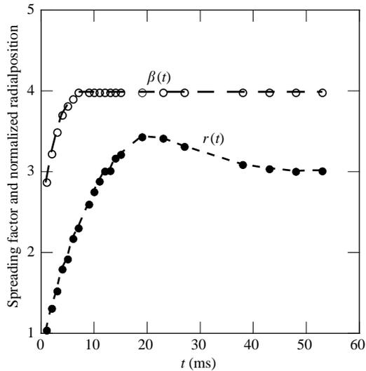
FIGURE 7. Time evolution of the spreading factor  $\beta(t)$  (open circles) compared to the normalized radial position of a test particle (filled circles) for suspension L2P2. The Reynolds number was  $Re_0 = 6500$  and the particle volume fraction was  $\phi = 0.02$ .
